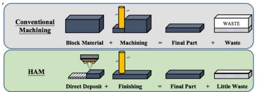
Figure 17. Comparison between conventional machining and hybrid process
