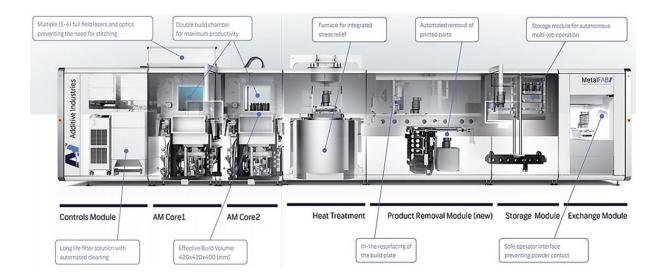
Figure 14. MetalFab1 system (Additive Industries) [52]
