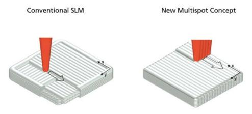
Figure 12. Comparison between conventional laser on SLM and multispot concept [50]
