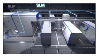
Figure 16. Automated powder transport (feed, extraction and recycling) from SLM Solutions
