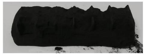
*Figure* 23: Example of an SLS part after the majority of bulk powder is removed
