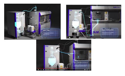
*Figure 13. Powder circulation through SLM machine system: (1) feed with virgin powder, (2) recirculate excess powder from overflow after manufacturing and (3) recover remnant powder from build chamber [51]*
